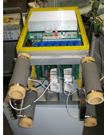
Figure 2: High Voltage Pulse Generator.
